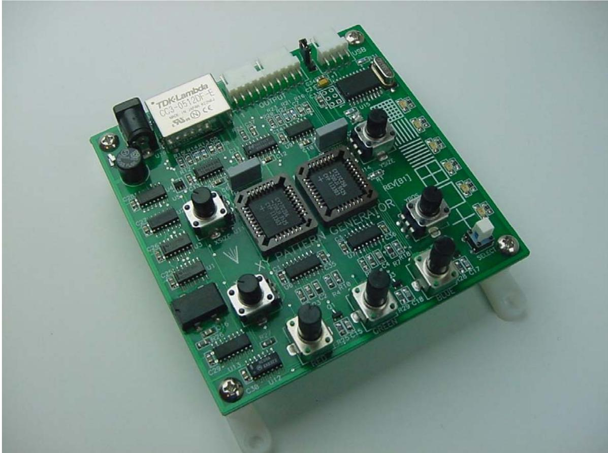
The X-Y Pattern Generator was designed as a test instrument to aid in the repair and alignment of B/W and Color X-Y monitors. This unit cannot be used on Raster scan monitors. The Pattern Generator comes equipped with pass through cable assemblies to fit Wells Gardner and Electrohome B/W and color X-Y monitors. The unit can be used on other X-Y monitors by building your own cables or ordering custom cables from [support@vector-labs.com](mailto:support@vector-labs.com)
