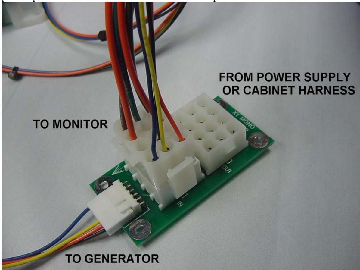
***MONOCHROME XY PASS THRU CABLE SHOWN AS EXAMPLE***
